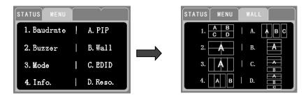
Press MENU+C (OUT3) + (1/2/3/4 or A/B/C/D) + Enter in sequence to select EDID for input channel. EDID options are: 3840x2160@60, 3840x2160@30, 1280x720@60, 1920x1080@60, 1366x768@60, 1920x1200@60, 1920X1080@30, 4096X2160@60
