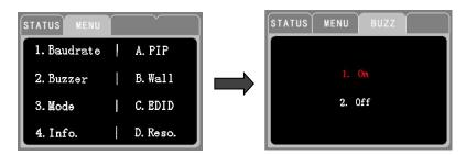
• Press MENU+3+(1/2)+ Enter in sequence to modify the display mode(matrix or video wall).
