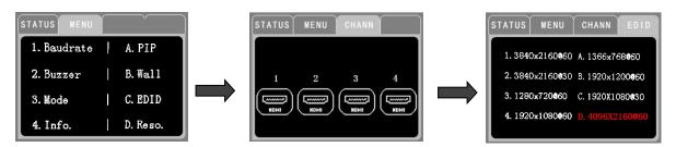
• Press MENU+D (OUT4) + (1/2/3/4 or A/B/C/D) + Enter in sequence to switch current HDMI output resolution: 3840x2160@60, 3840x2160@30, 1280x720@60, 1920x1080@60, 1366x768@60, 1920x1200@60, 1920X1080@30 , 4096X2160@60
