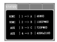
The left column indicates the current audio input format (HDMI is embedded audio, AUX is analogue audio) and the middle part indicates the input and output corresponding status. The right column indicates the current resolution of the corresponding output port.
